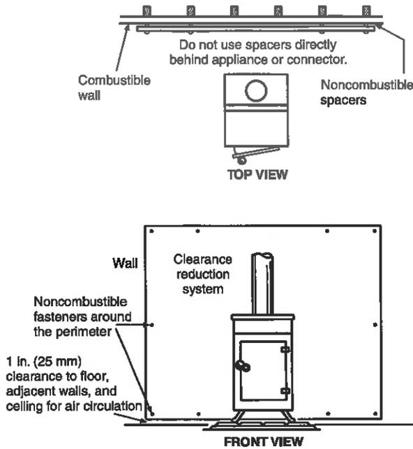
**FIGURE 13.6.2.1(a) Clearance Reduction System — Fastener Location.**
