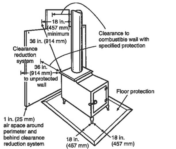
**FIGURE 13.6.2.1(b) Distance to Combustible Wall/Floor.**
