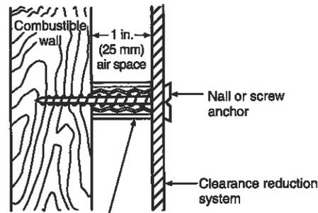
1 in. (25 mm) noncombustible spacer such as stacked washers, small-diameter pipe, tubing, or electrical conduit
